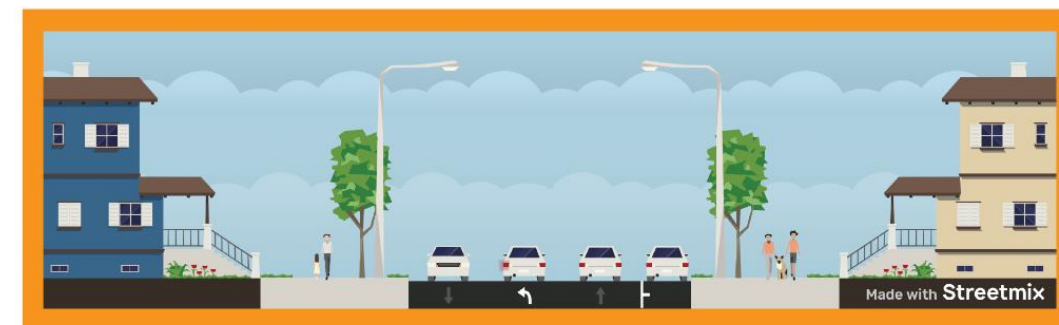
Three lane (with center turn lane) with limited parking
